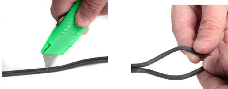
5. Take the fan wire that is provided. **The wires are already prepped and should not be cut off.** If you do the cut the wires, then you will need to strip 1 inch of wire insulation from fan connector wire and twist the copper back onto itself over the insulation on each side. This is important to make sure that there will be a proper connection.
