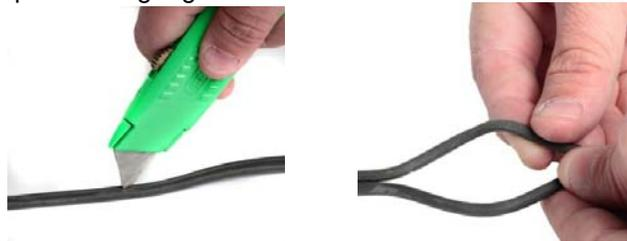
5. Take the fan wire that is provided. **The wires are already prepped and should not be cut off.** If you do cut the wires, then you will need to strip 1 inch of wire insulation from fan connector wire and twist copper back onto itself over the insulation on each side. This is important to make sure that there will be a proper connection.
