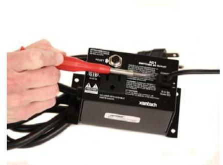
5. Plug the dehumidifier into the relay kit. Plug relay kit into available electrical outlet.
