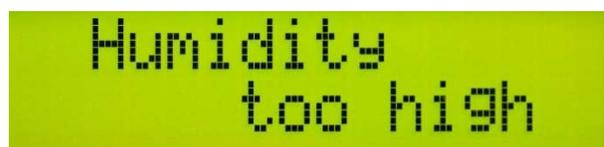
The humidity alarm setting is defaulted to the off position, so it may not be active on your system. This feature can be turned on to alert you anytime the crawlspace exceeds a set internal relative humidity level. It can be set anywhere between 73-98%, in increments of 5%. See Section 10.5.5 for alarm settings.
