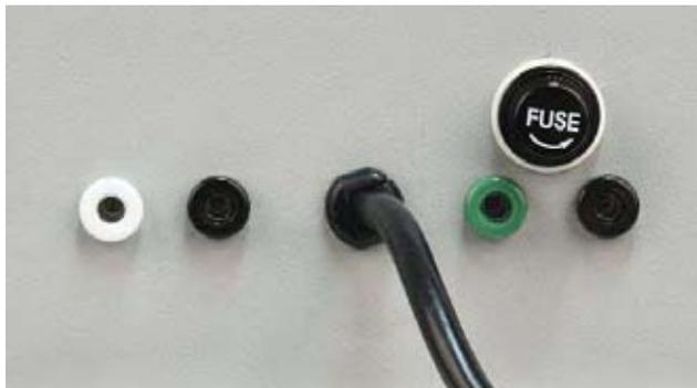
If your ATMOX System has been equipped with the option to use a battery connection, the bottom of the EZ Controls power supply box will have green and black plugs on bottom right side along with a Fuse.
