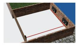
2 Begin at the controller and start taking the primary wire to the components. At the end of a run, cut off any wire.
