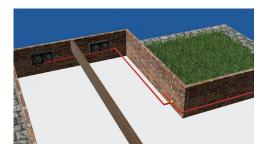
If extra length is needed on the primary wire, attach a supplemental wire to the primary wire to keep going in the same direction.
